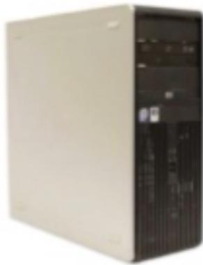
The computer case is the metal and plastic box that has all the parts in it that make the computer work. These are called the motherboard, central processing unit (CPU) and power supply. The front of the case usually has an On/Off button and this is when you switch your computer on or off.
